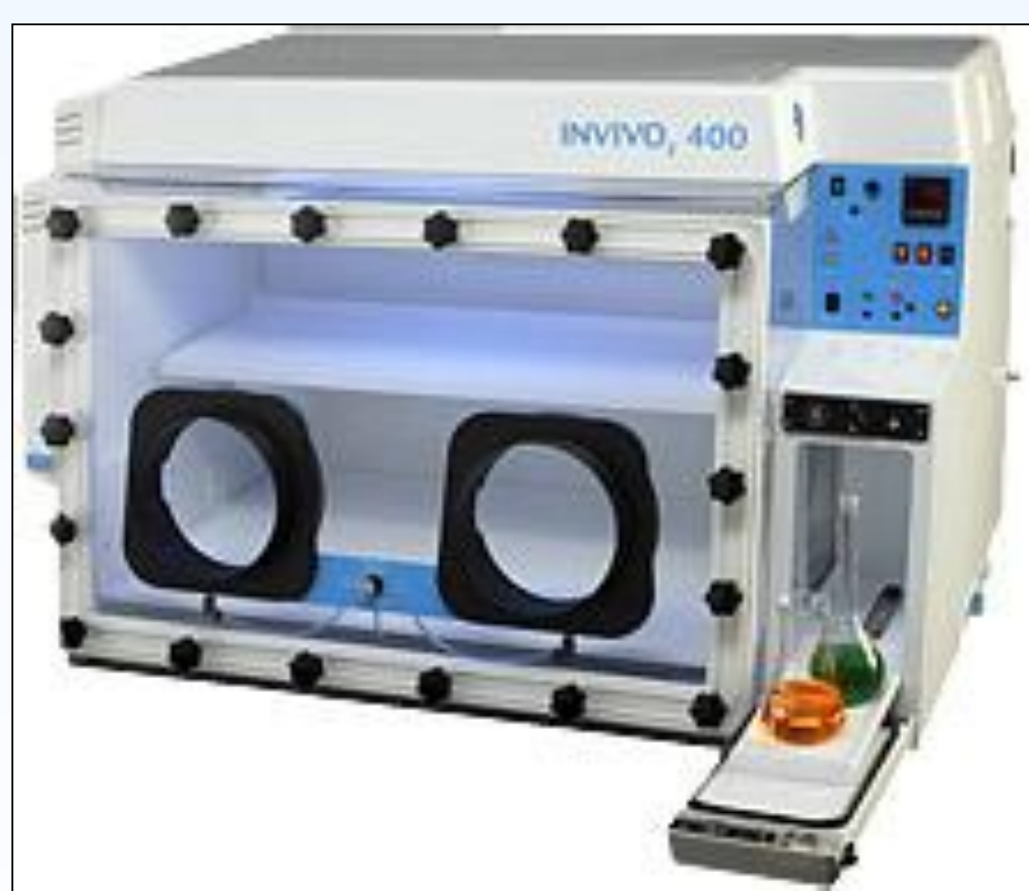
Figure 1: For experiments in hypoxia, a Invivo 400 from Ruskinn Technology was used.
